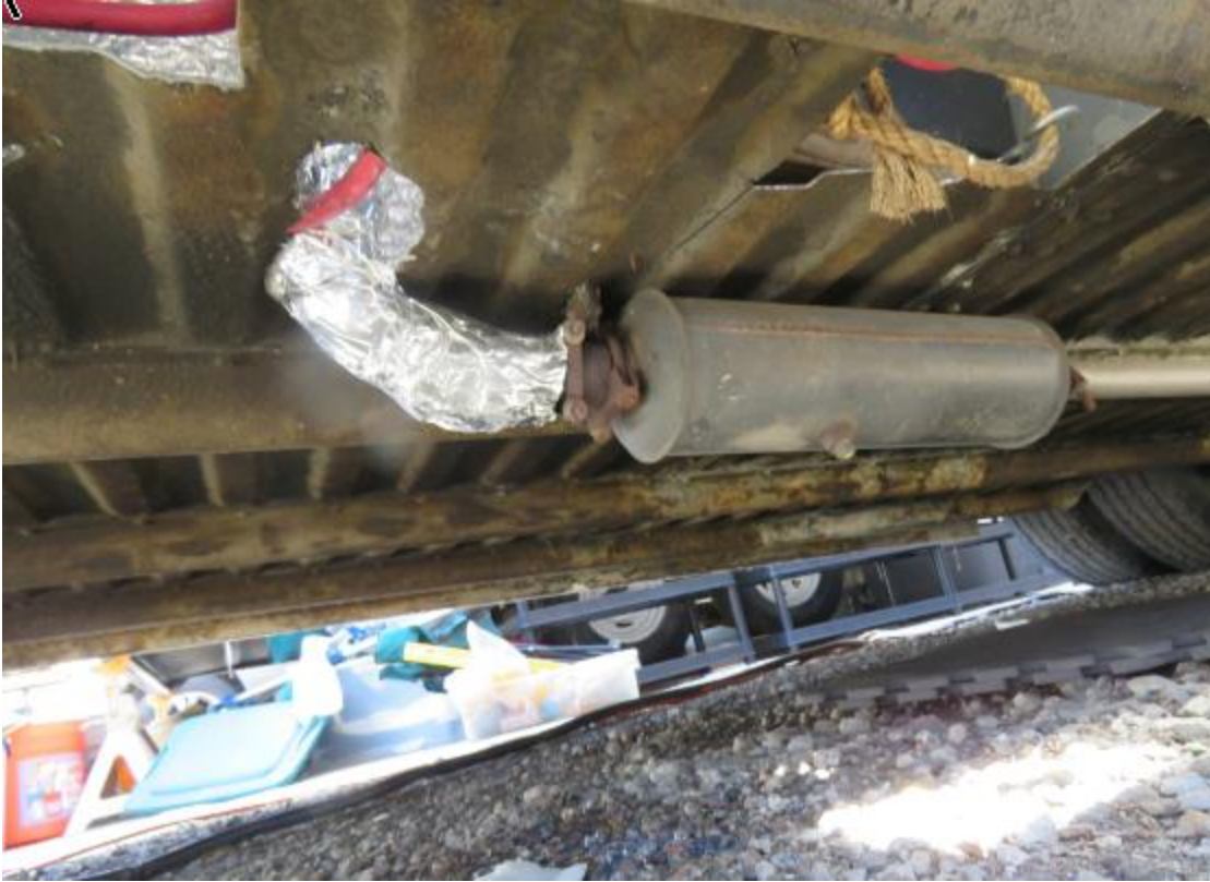
Wrap under the bus up to the muffler.
